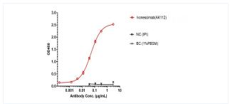
Ivonescimab bound to PD-1 protein, and then rebounded to secondary antibodies (Anti-human-IgG-Fc-HRP) , and read OD450. As shown in fig , Ivonescimab bound to huPD-1-His, and the EC50 was  $0.051\ nM$ .
