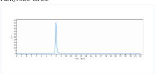
The purity of Anti-cMet & EGFR Reference Antibody (Emb01) is 97.60% , determined by SEC-HPLC.
