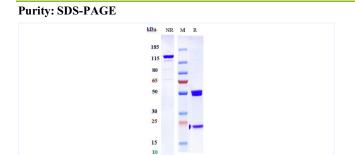
Anti-ANG2 & VEGFA Reference Antibody (Vanucizumab) on SDS-PAGE under reducing (R) condition. The purity of the protein is greatethan 96%.
