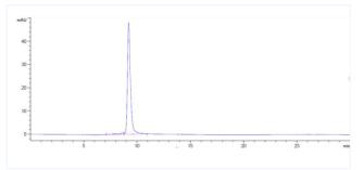
The purity of Anti-TREM2 (Py314) is 97.69%, determined by SEC-HPLC.
