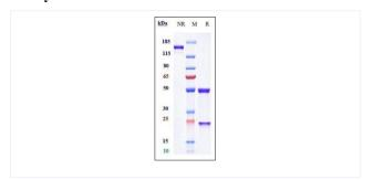
Anti-GD2 (naxitamab) on SDS-PAGE under reducing (R) condition. The purity of the protein is greater than 95%.
