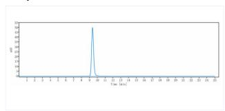
The purity of Anti-GD2 (naxitamab) is 100.00 %, determined by SEC-HPLC.
