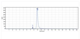
The purity of Anti-Tau (zagotenemab) is 98.97%, determined by SEC-HPLC.
