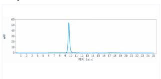
The purity of Anti-Integrin a4b7 (ITGA4 & ITGB7) (vedolizumab) is 100%, determined by SEC-HPLC.
