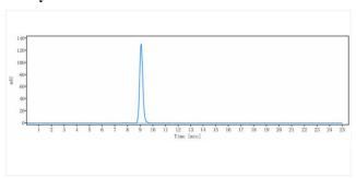
The purity of Anti-TNFSF13B / BAFF / CD257(tabalumab) is more than 95%, determined by SEC-HPLC.
