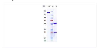
Anti-TNFSF13B / BAFF / CD257 (tabalumab) on SDS-PAGE under reducing (R) condition. The purity of the protein is greater than 90%.
