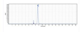
The purity of Anti-TBFbR2 (LY3022859) is98.25%, determined by SEC-HPLC.
