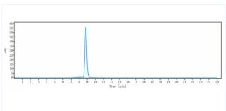
The purity of Anti-Amyloid Beta (solanezumab)is 96.84%, determined by SEC-HPLC.
