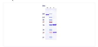
Anti-NaPi2b / SLC34A2 (upifitamab) on SDS-PAGE under reducing (R) condition. The purity of the protein is greater than 95%.
