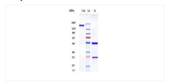
Anti-PDCD1 / PD-1 / CD279 (sintilimab) on SDS-PAGE under reducing (R) condition. The purity of the protein is greater than 95%.
