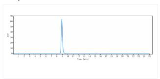
The purity of Anti-PDCD1 / PD-1 / CD279(cetrelimab) is more than 95%, determined by SEC-HPLC.
