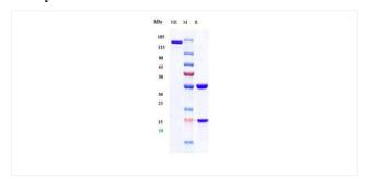
Anti-PDCD1 / PD-1 / CD279 (cetrelimab) on SDS-PAGE under reducing (R) condition. The purity of the proteinis greater than 90%.
