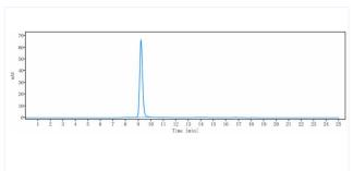
The purity of Anti-PDCD1 / PD-1 / CD279(prolgolimab) is more than 95%, determined by SEC-HPLC.
