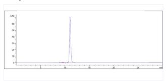
The purity of Anti-NT5E / CD73 (uliled limab)is 98.34%, determined by SEC-HPLC.
