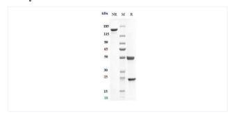
Anti-Integrin aL / ITGAL / CD11a (efalizumab)on SDS-PAGE under reducing (R) condition. The purity of the protein is greater than 95%.
