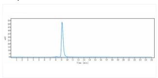
The purity of Anti-Integrin aL / ITGAL / CD11a(efalizumab) is 98.77%, determined by SEC-HPLC.
