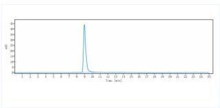
The purity of Anti-FcRn (FCGRT & B2M)(nipocalimab) is 100%, determined by SEC-HPLC.
