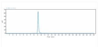
The purity of Anti-IGF1R / CD221(lonigutamAb) is 100%, determined by SEC-HPLC.
