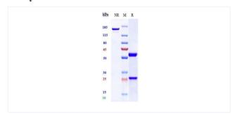
Anti-TSPAN26 / CD37 (lilotomab) on SDS-PAGE under reducing (R) condition. The purity of the protein is greater than 95%.
