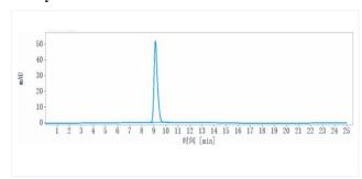
The purity of Anti-TSPAN26 / CD37(lilotomab) is 100%, determined by SEC-HPLC.
