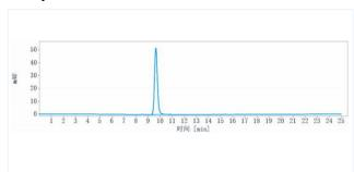
The purity of Anti-MUC17 (Forerunner patentanti-Muc 17) is more than 95%, determined by SEC-HPLC.
