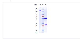
Anti-IL-6 / IFNb2 (elsilimomab) on SDS-PAGE under reducing (R) condition. The purity of the protein is greater than 95%.
