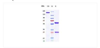
Anti-SOST / Sclerostin (blosozumab) on SDS-PAGE under reducing (R) condition. The purity of the protein is greater than 95%.
