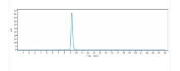
The purity of Anti-TFPI (befovacimab) is morethan 95%, determined by SEC-HPLC.
