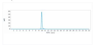
The purity of Anti-B7-H1 / PD-L1 / CD274(garivulimab) is more than 95%, determined by SEC-HPLC.
