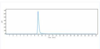
The purity of Anti-CCR5 / CD195 (leronlimab) is more than 95%, determined by SEC-HPLC.
