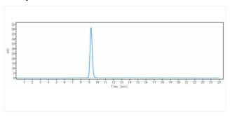
The purity of Anti-SCN11a / Nav1.9 (Wuhan U.patent anti-Nav1.9) is more than 95%, determined by SEC-HPLC.
