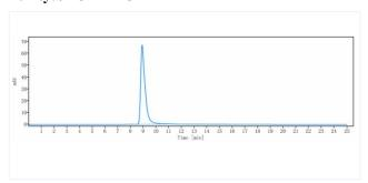
The purity of Anti-CD3e (teplizumab) is 100%, determined by SECHPLC.
