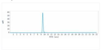
The purity of Anti-SLC44A4 (ASG-5ME) ismore than 95%, determined by SEC-HPLC.
