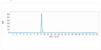
The purity of Anti-Complement C2(ARGX-117) is 100%, determined by SEC-HPLC.
