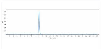
The purity of Anti-IFNAR1 (anifrolumab) is 98.75%, determined by SEC-HPLC.
