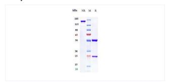
Anti-IFNAR1 (anifrolumab) on SDS-PAGE under reducing (R) condition. The purity of the protein is greater than 95%.
