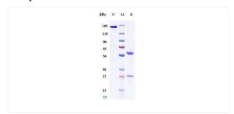
Anti-PVRIG (GSK4381562) on SDS-PAGE under reducing (R) condition. The purity of the protein is greater than 90%.
