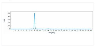
The purity of Anti-MIF (imalumab) is more than 95%, determined by SEC-HPLC.
