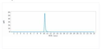
The purity of Anti-IL-1RL2 / IL-36R (spesolimab) is more than 95%, determined by SEC-HPLC.
