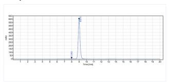
The purity of Anti-IL-1R1 / CD121a (AMG108) is 99.03%, determined by SEC-HPLC.
