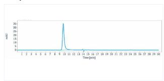
The purity of Anti-IDO2 (LIMR patentanti-IDO2) is 97.85%, determined by SEC-HPLC.
