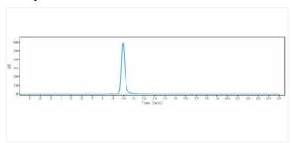
The purity of Anti-GIPR (Amgen patentanti-GIPR) is more than 95%, determined by SEC-HPLC.
