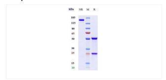
Anti-CD200 (samalizumab) on SDS-PAGE under reducing (R) condition. The purity of the protein is greater than 95%.
