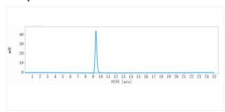
The purity of Anti-RGMA (elezanumab) is 100%, determined by SEC-HPLC.
