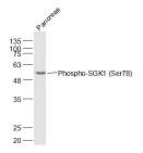
Sample: Pancreas (Mouse) Lysate at 40 ug Primary: Anti-Phospho-SGK1 (Ser78) (bs-3395R) at 1/1000 dilution Secondary: IRDye800CW Goat Anti-Rabbit IgG at 1/20000 dilution Predicted band size: 49 kD Observed band size: 50 kD
